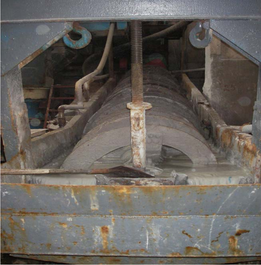
Figure 5: Spiral Classifier at Jiaojia Gold Mine
